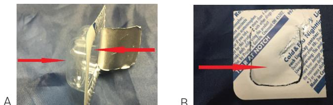
**Figure 2.** The blister pack areas of cold and flu liquid cap medications that were measured by FTIR: (A) the inside and outside of the clear polymer blister and (B) the unprinted region of the outer foil (lidding).
