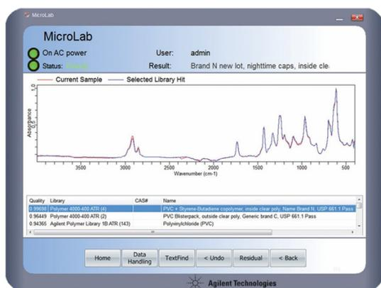
**Figure 9.** The FTIR ATR library search result from the Cary 630 FTIR MicroLab software. The unknown sample (red spectrum) is a blister polymer. A search was undertaken against a library of known USP chapter <661.1> polymers created from name brand and generic blisters. The top hit is a near-perfect match (quality 0.99698) to the library material, PVC and SBR copolymer (blue spectrum).
