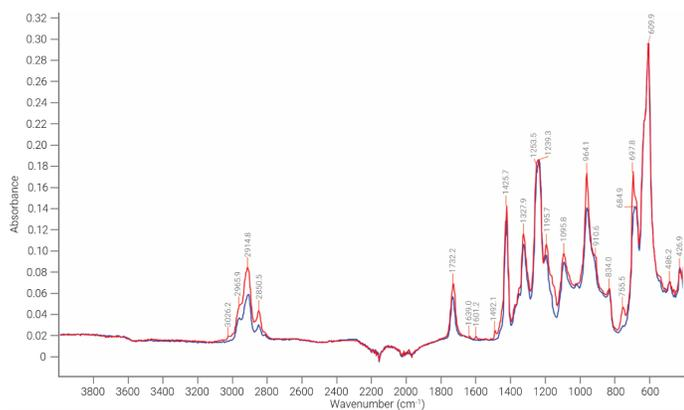
**Figure 4.** The FTIR spectral overlay of the PVC outer blister layer of a generic product (blue) overlaid with the inner blister layer of a name brand product (red), indicating PVC with additional SBR copolymer in the name brand material.
