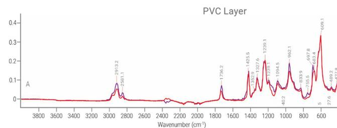
**Figure 3.** FTIR spectra of clear blister polymers from over-the-counter cold medicines collected on a Cary 630 FTIR with diamond ATR module. The outer blister layer of a generic product (red) is overlaid with the inner blister layer of a brand name product (purple). The band at  $1736\text{ cm}^{-1}$  indicates the presence of  $\sim 2\text{--}3\%$  of a copolymer such as polyacrylate or polyvinylacetate.
