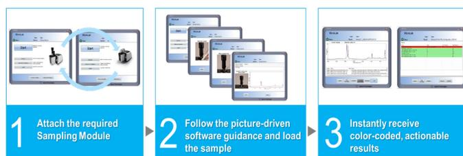
**Figure 1.** The MicroLab software for FTIR analysis automatically recognizes the attached sampling module and applies the correct parameters. The software navigates the user, step by step, through the analytical workflow using instructive pictures. Color-coded results, directly reported after data acquisition, make data review quick and intuitive.
