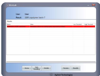
**Figure 5.** MicroLab software automatically calculates the SBR content of packaging material samples. Color-coded, actionable results are reported directly after data acquisition in line with the threshold settings of the method.
